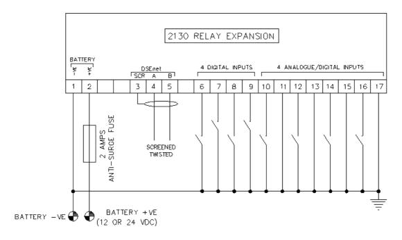
NOTE: Configuration of the inputs is performed in the host controller. The 4 analogue inputs can be reconfigured to be digital inputs if required and connected as shown above.
