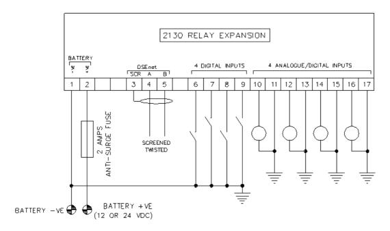
2130 SHOWN CONNECTED AS 8 DIGITAL INPUTS
