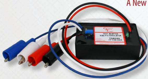
The TSE050 simulates a running engine when connected to the magnetic pickup input on a speed control. An on-board potentiometer allows the signal to be adjusted between 750 to 10,000 Hz and is compatible with all GAC speed controls using a magnetic pickup.
