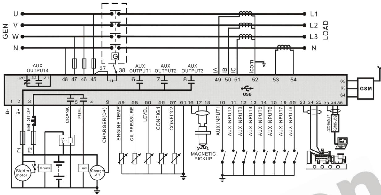
HGM9310MPU(CAN) typical application diagram
